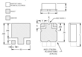
Note 1 - Additional plated thru holes will be provided on this edge, as space allows.
