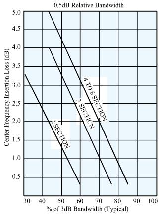
It is often advantageous to know more about the passband of a filter than its center frequency loss and its 3dB bandwidth.
