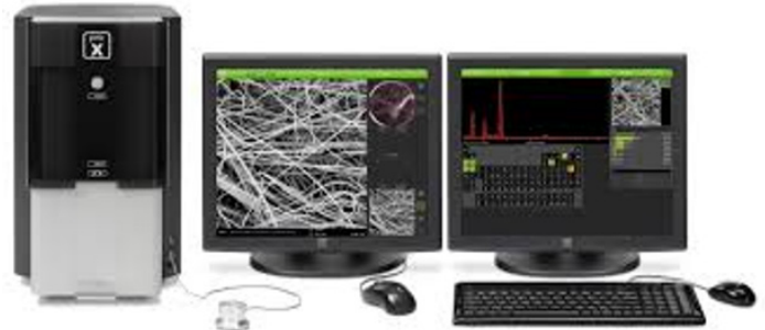
Figure 5. This SEM/EDX system provides 130,000 \times total magnification with 10-nm feature resolution, a built-in EDX, and BSE detector in support of surface and metallurgical analysis in
