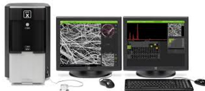
Figure 5. This SEM/EDX system provides 130,000 \times total magnification with 10-nm feature resolution, a built-in EDX, and BSE detector in support of surface and metallurgical analysis in
