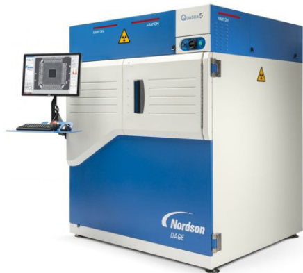
Figure 4. A three-dimensional (3D) x-ray system with computer tomography provides a total magnification of 45,000 \times for nondestructive FA with 350-nm feature resolution of cracks and faults.
