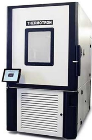
Figure 1. An essential tool for FA is a temperature/humidity chamber with wide control ranges.
