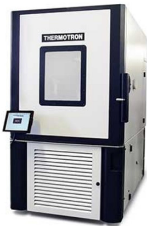
Figure 1. An essential tool for FA is a temperature/humidity chamber with wide control ranges.
