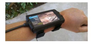
Rugged glass resistive touch screen technology is combined with an HD, sunlight-readable display enabling a portable, man worn or handheld display. The device provides a crisp, full-color, interactive wearable in a completely sealed form factor for use in adverse environments. A single cable, carrying video, power, and touchscreen input data, connects the wrist displayto any Windows-based computer.
