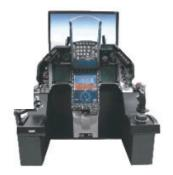
The F-16 desplay, designed to replace several legacy analog instruments with one glass, digital cockpit unit. Designed with a custom cut, hardened and laminated glass, the new multifunction display features configurable bezel buttons.
