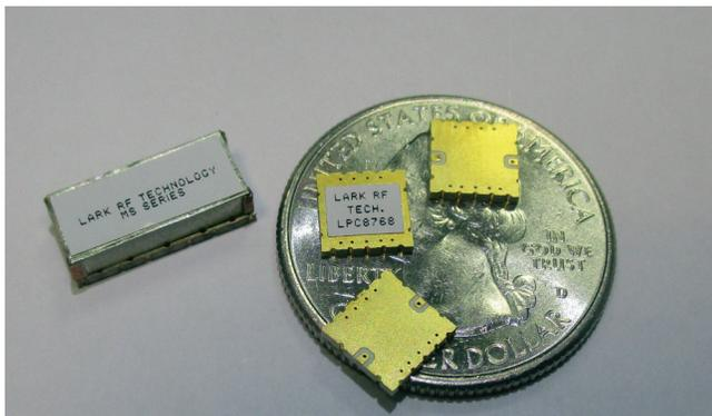
Fig. 4 Switched filter bank showing stacking LCP BP filters
