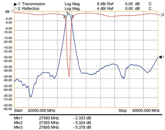
Fig. 1 Fused Silica SMT BP filter:
