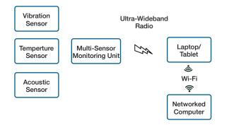
using sound, vibrations, and temperature. The MSMU connects to several commercially available sensors. The solution works by using a phased array that directs the signal precisely, rather than relying on a broad emitting signal that may lead to inaccurate data.
